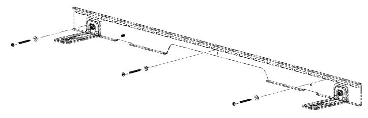
INSTALL AND TIGHTEN APPROPRIATE SCREWS USING PROVIDED FLAT WASHERS.
